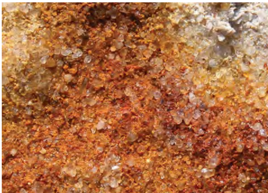
Sand grains (visible as individual quartz grains) coated and bridged with illuvial clay (smooth yellowish color). (Photo courtesy of John Kelley)
